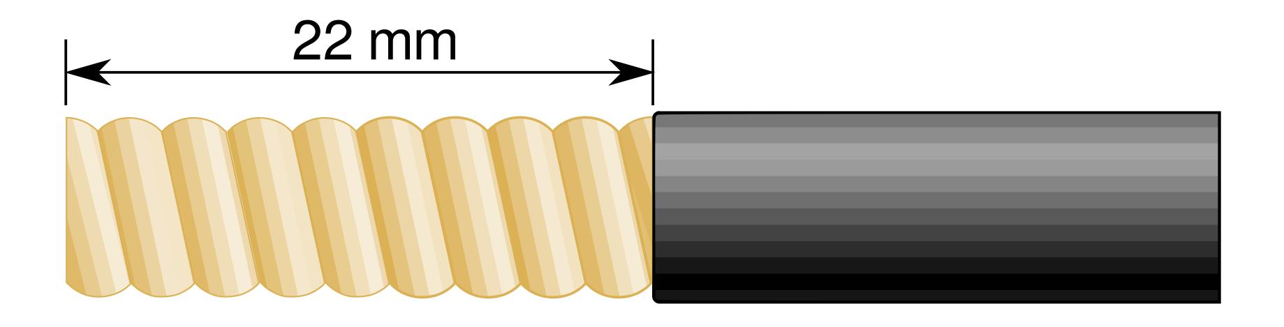
Using a sharp knife, remove 10mm of the copper screen and dielectric. Clean all copper surfaces with an alcohol wipe.
